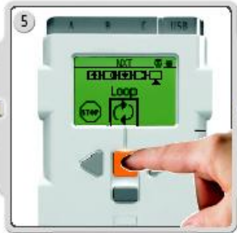
Now select if you want the program to Loop. This means that the program will run again and again until you switch off the NXT. For our little test, select Loop.
