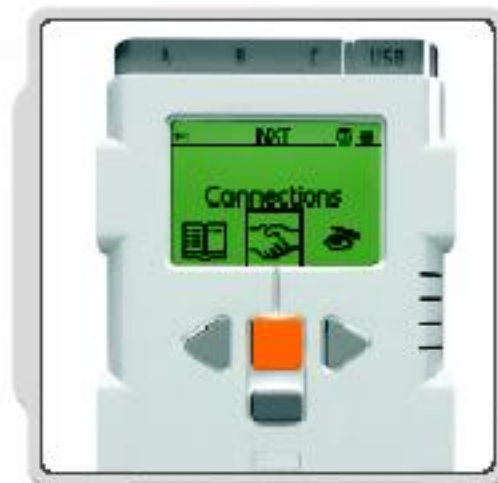
Connections This item displays your current connections. You can connect your NXT to three devices at the same time (on Line 1, 2 and 3), while one device can connect to you (on Line 0). Note, however, that while you can be "connected" to up to three devices, you can only "communicate" with one device at a time.
